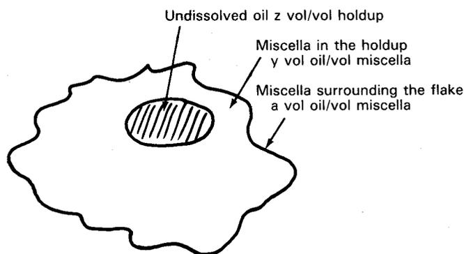
FIG. 2. Schematic flake with derivation of extraction rate equation. Let  $r$  be the total oil in the flake, vol oil/vol holdup.  $\therefore r = y(1 - z)$ . For 1 kg flakes, oil content is 0.788 l. In time  $dt$ :  $0.788dr = -k(y - a)dt$  where  $k$ , is a constant whose dimensions are  $l/kg \text{ min}^{-1}$ . Let  $k = k_1/0.788$ .  $\therefore dr = -k(y - a)dt$ .
