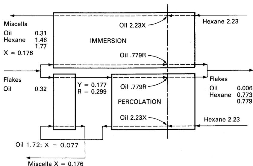
FIG. 3. Oil and hexane volumes balance in continuous extraction. Basis, 100 kg meats. Volumes in liters.
