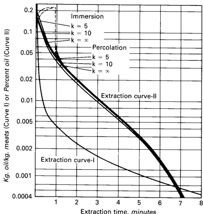
FIG. 4. Curve 1, residual oil vs. extraction time from batch laboratory extraction of 0.008" thick soybean flakes with hexane. Curve 2, predicted miscella concentrations vs. extraction time in continuous extractors.
